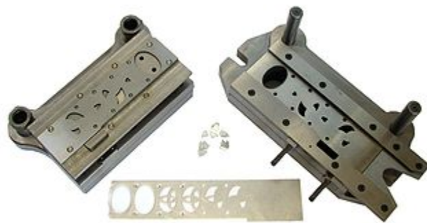
Progressive die with scrap strip and stampings
