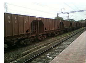
BOBRN class hopper cars freight rakes used by Indian Railways
