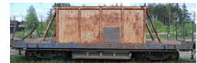
Kambarka Engineering Works hopper car to transport track ballast, 750 mm (2 ft 5½ in) gauge
